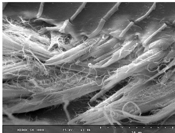
Figure 1: Biopolymeric fibers (collagen) from a cross-sectional view of Oreochromis niloticus scale
